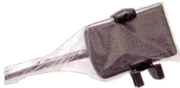
Figure 17: Using protective sensor sheath
